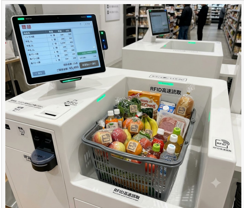
Customer has placed entire contents of cart in the AsReader Reading Tub for easy self checkout
