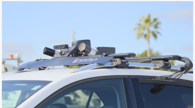
Noteworthy AI's Inspect Edge Camera on Utility Fleet Vehicle Roof
