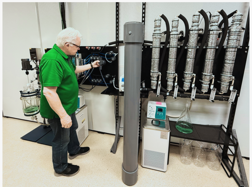
Brian J. Andrew, President, CEO, and co-founder of Precision Periodic, stands beside the company's demonstration Multi-Scale Refining Unit (MSRU) and a full-scale column used for size reference in scaling to commercial production.
