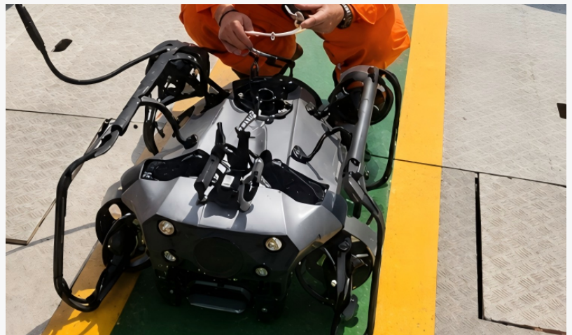
INMARVENCO deploys the CHASING X Industrial ROV for an offshore oil platform inspection in Venezuela.
