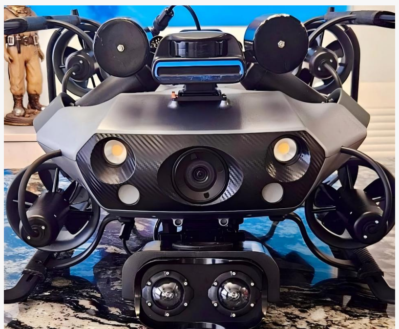
The CHASING X was configured with 3D scanning, sonar, ultrasonic thickness measurement and cathodic protection inspection technologies.
