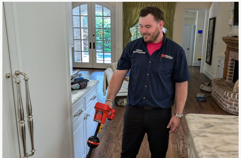
Non-invasive acoustic leak detectors find slab leaks without digging.
