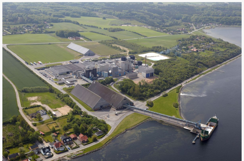
Dansk Salt's fully electrified salt production facility in Marriager, Denmark. During the initial charging of the cavern with compressed air, the brine currently stored within the cavern, will be released to the plant, generating highly pure salt
