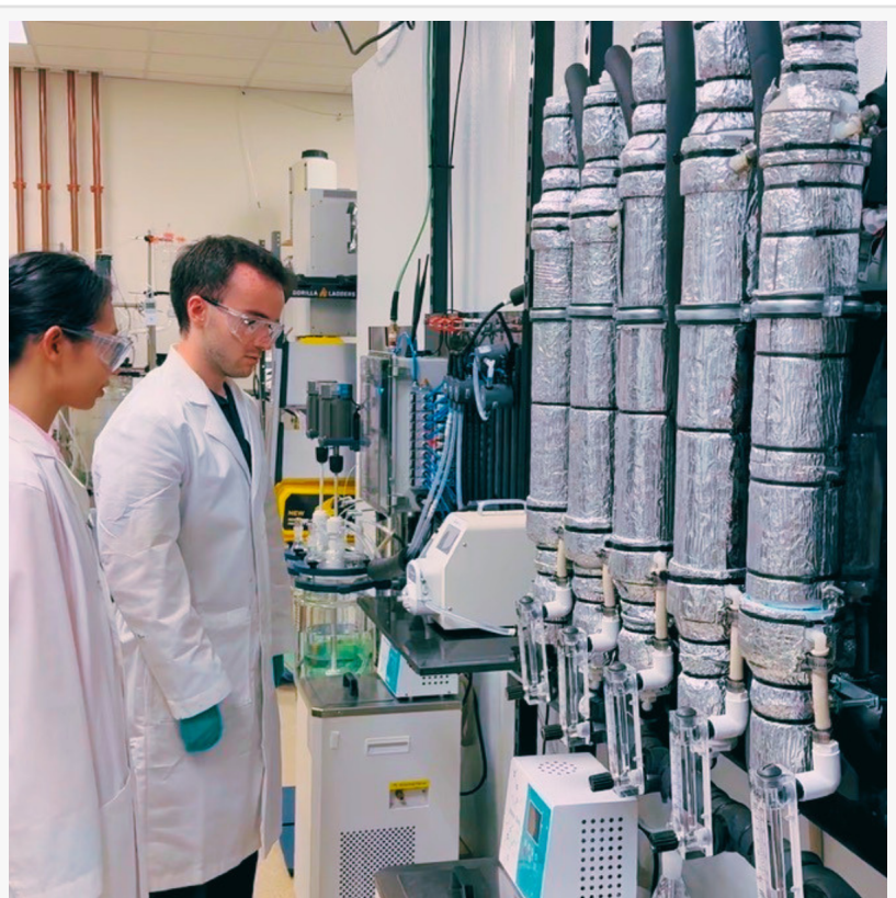
Precision Periodic's 1/10th scale Multi-Scale Refining Unit (MSRU) demonstrates the modular, clean-process technology that will scale to full production at the Florida facility, converting nickel mixed hydroxide precipitate into battery-grade materials.
