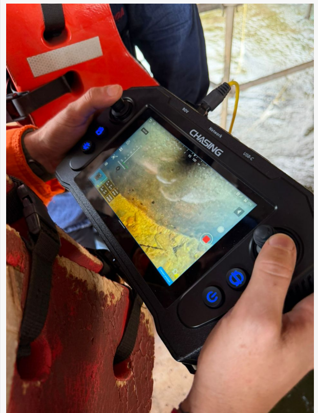
An operator monitors live underwater video from CHASING X during the Caroní River pile scour inspection in strong-current, low-visibility conditions.
