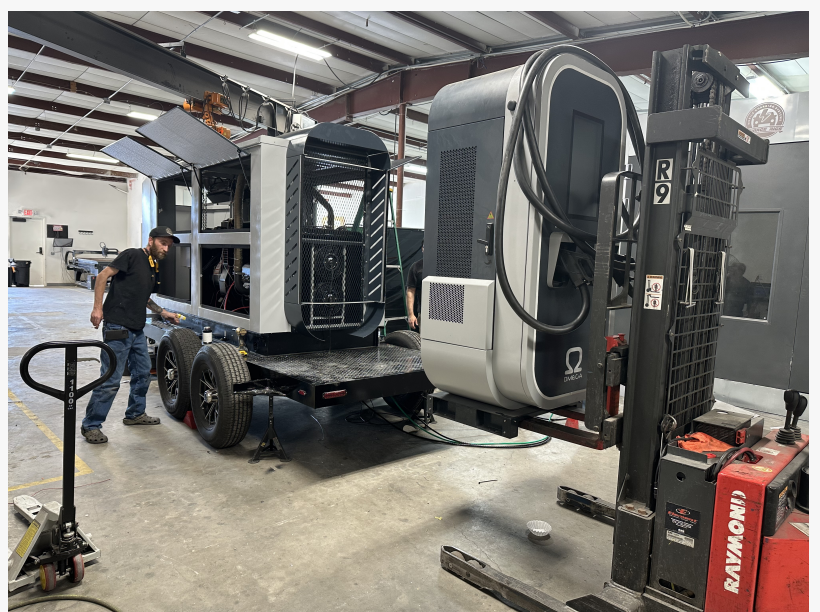
Custom Mobile Charger Buildout
