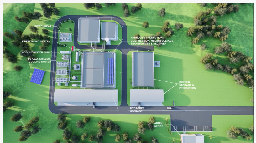
Visual Illustration of Aternium's Hydrogen Production Facility
