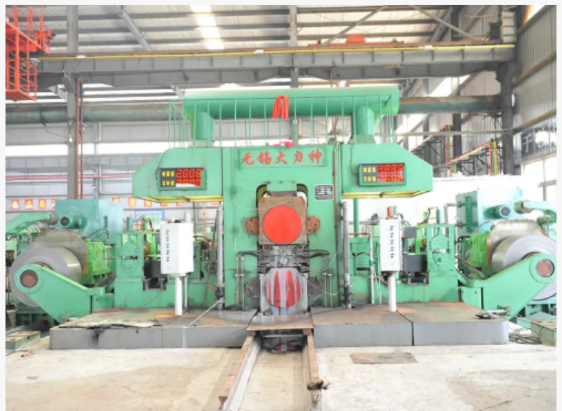
Cold Rolling Mill
