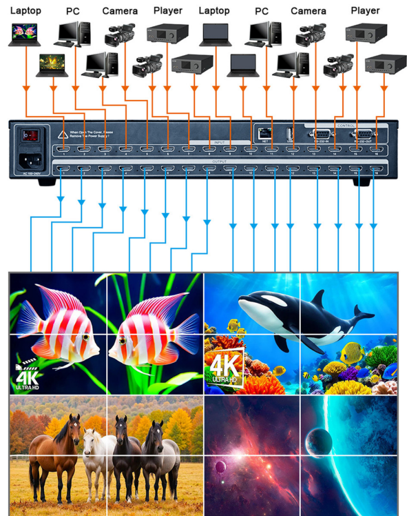
Multi-mode 4K 30 Hz HDMI Switch
