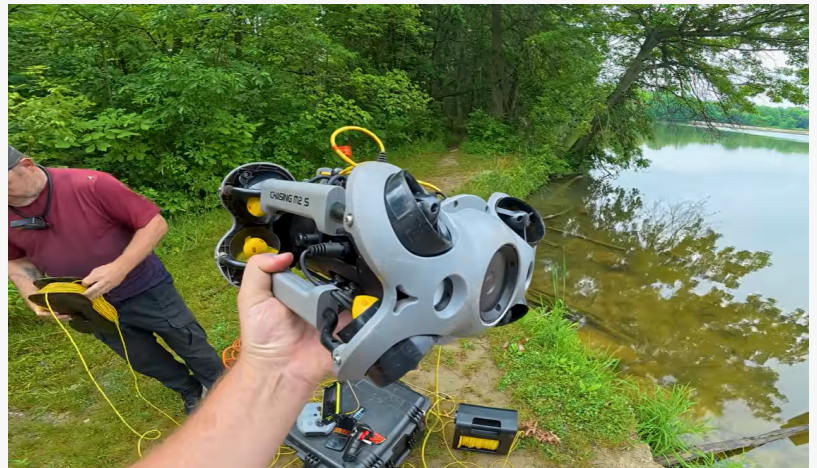
The search team deploys the compact CHASING M2 S underwater ROV directly from the shoreline to visually inspect the sonar target.
