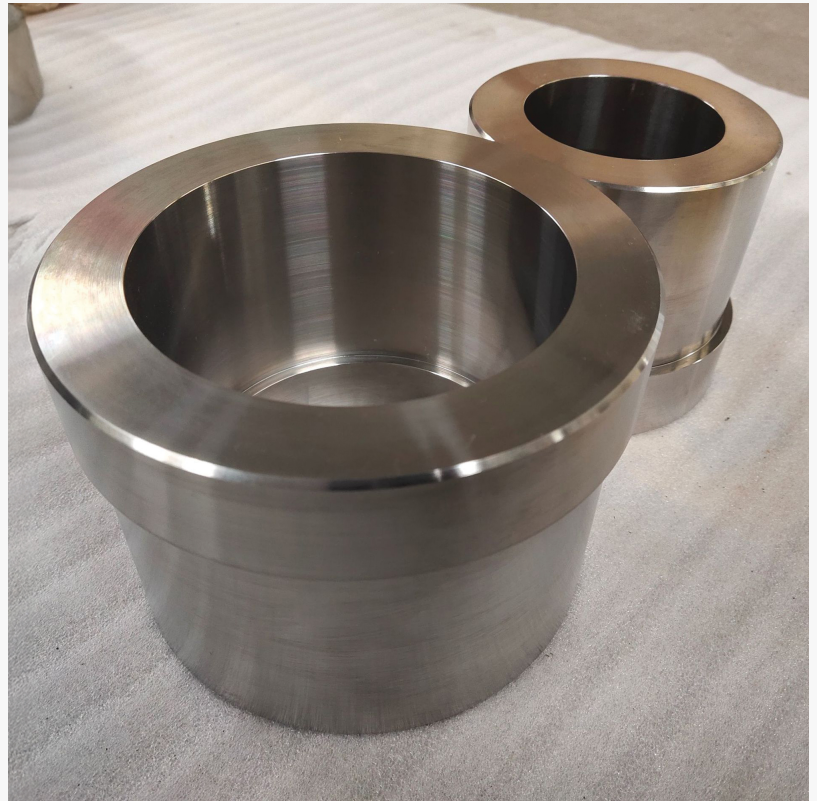
All parts are rough machined to 250 RMS or better.
