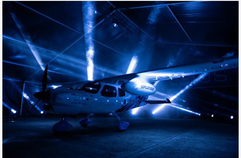
The H2-Sling, Switzerland's first hydrogen-powered aircraft, developed by Cellsius at ETH Zurich. Source: Cellsius
