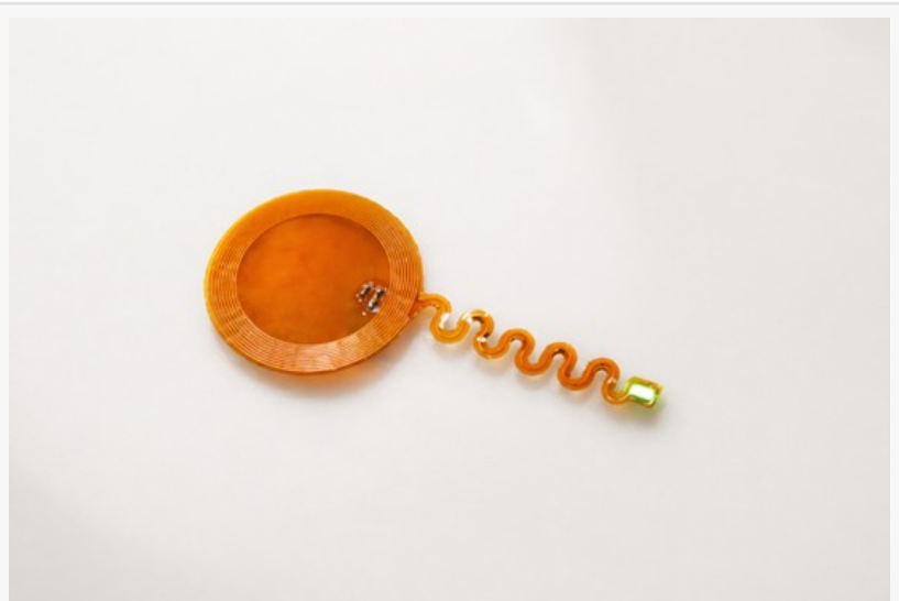
The wireless implantable flexible microsystem developed in this study to enable localized light delivery for photodynamic therapy.
