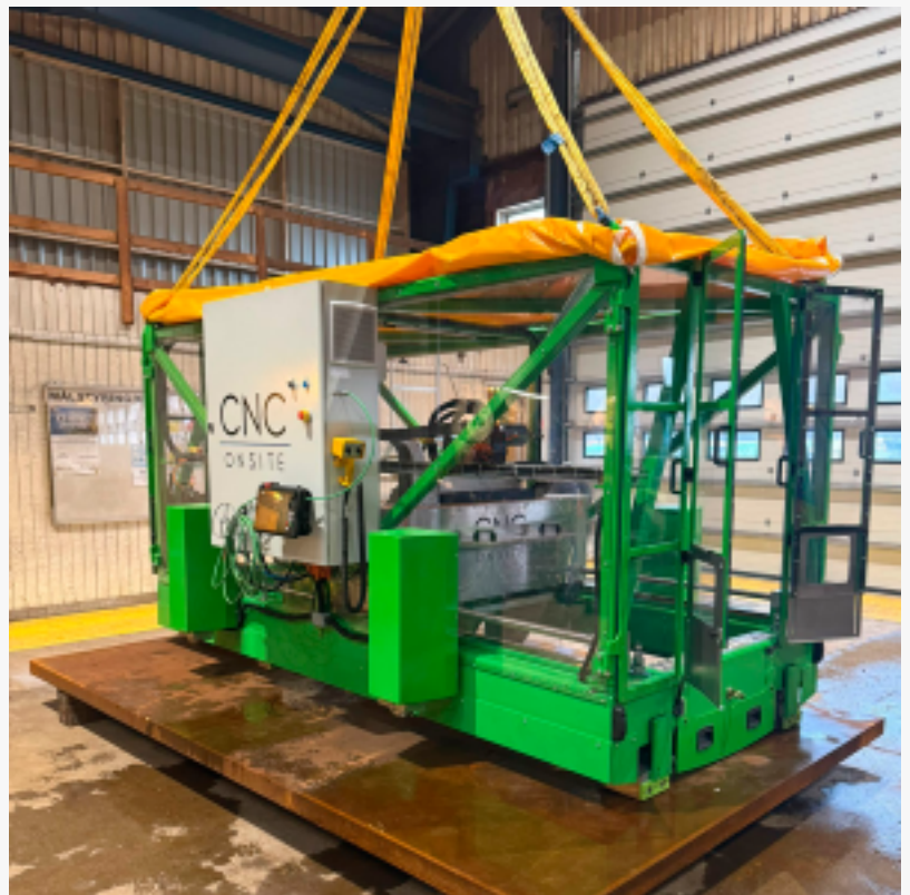
CNC Onsite's mobile 4-axis gantry milling machine prepared for lifting and transport at the facility in Aalborg.
