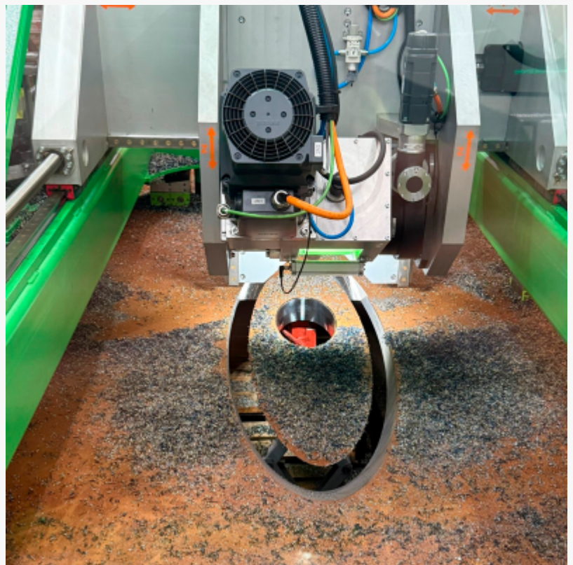
CNC Onsite's milling machine performing a 45-degree angled cutout for a cable penetration hole.
