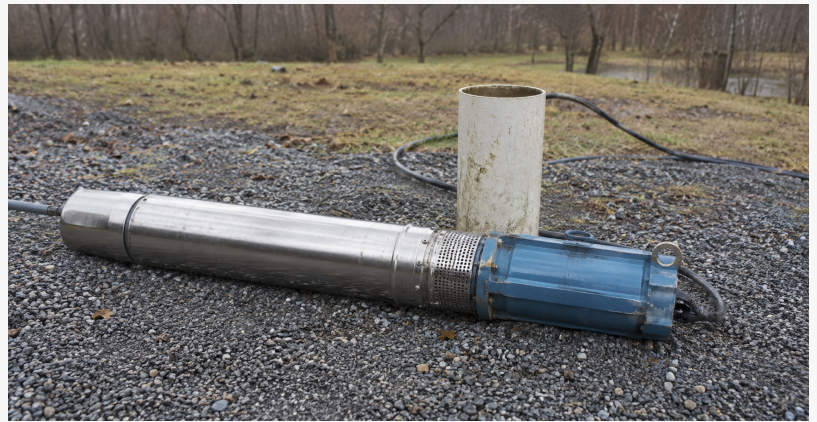
Submersible well pump and motor assembly beside an open well casing in a rural yard.
