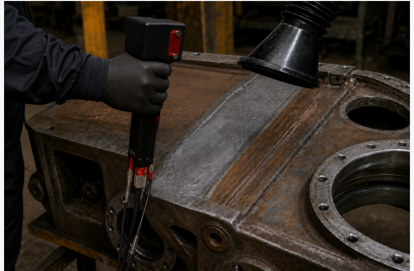
AI-generated close-up illustrating one-handed laser rust removal with the cleaning head positioned away from the metal surface and a fume-extraction hood located near the work area.
