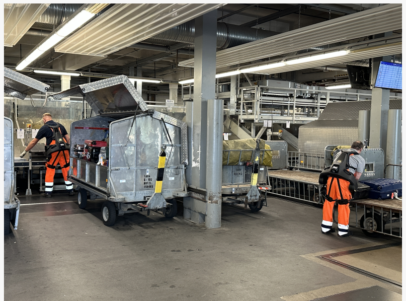
Human-centric robotics at Nuremberg Airport: AI-powered exoskeletons support baggage handlers in physically demanding lifting and moving tasks.
