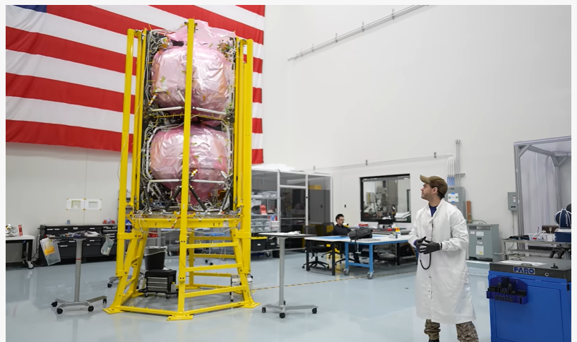
The Scorpius Space Launch Companies' PRESSURMAXX propulsion system.
