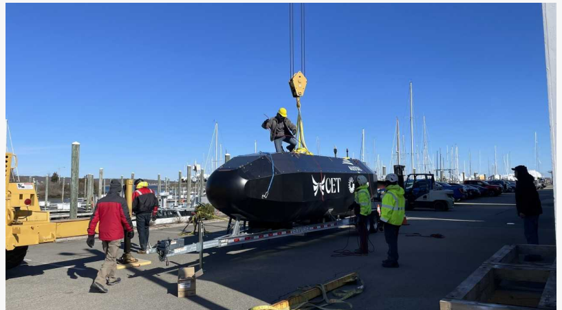
CET team members prepare the HADALUS autonomous underwater vehicle for launch.
