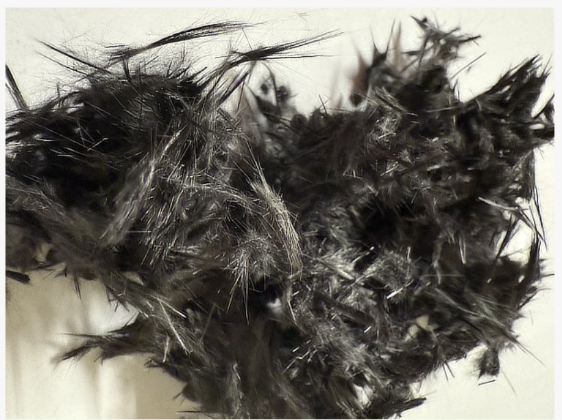
24mm Liberated rCF from Pyrolysis
