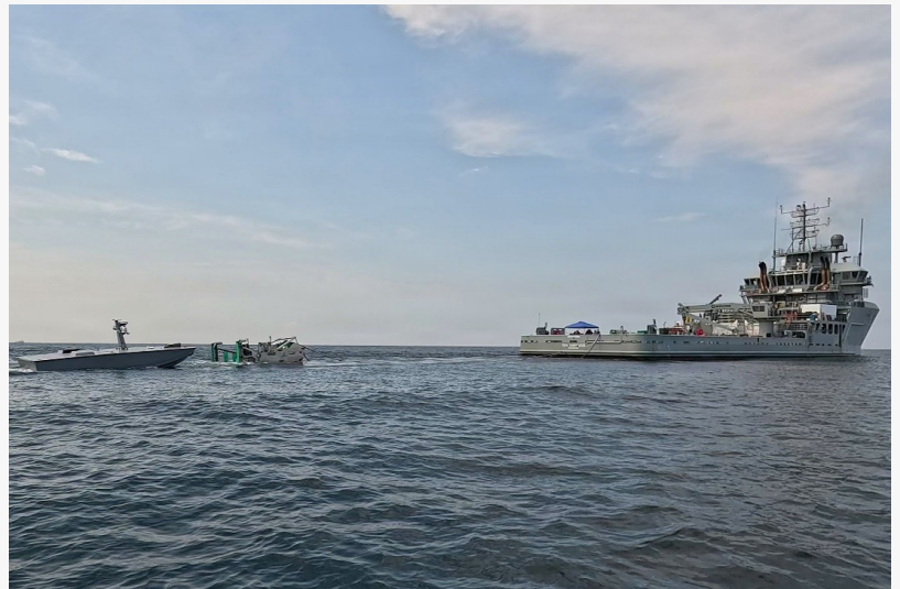
A MARTAC Devil Ray T38 is Autonomously Refueled At-Sea
