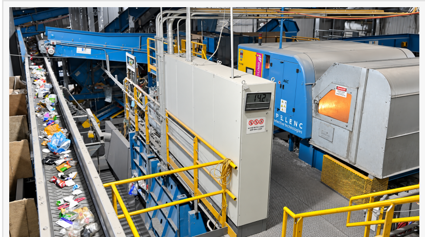
PELLENC optical sorting equipment at a California Waste Solutions recycling facility
