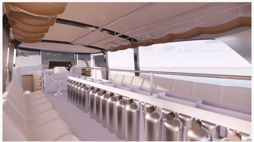
Rendering of the AT40 Dive main deck, with kit-up seating either side and centreline tank racks.
