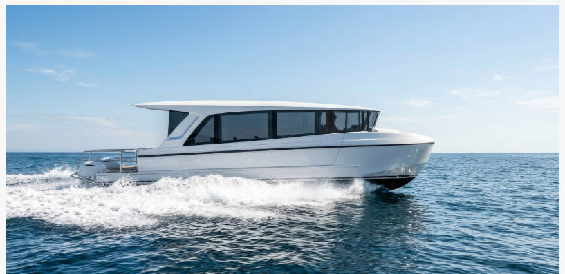
Rendering of the AT40 underway at cruising speed. All three versions share the same 12.99 metre (42.6 ft) hull.
