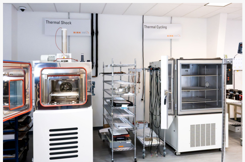
Thermal shock and thermal cycling test stations.
