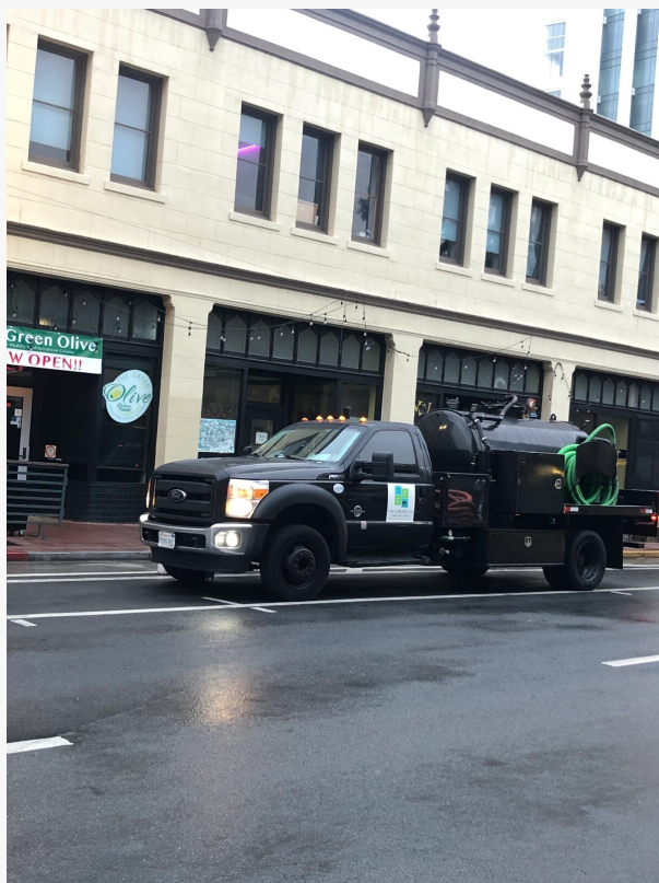
Grease management company service truck used for commercial grease trap pumping and interceptor cleaning in Los Angeles
