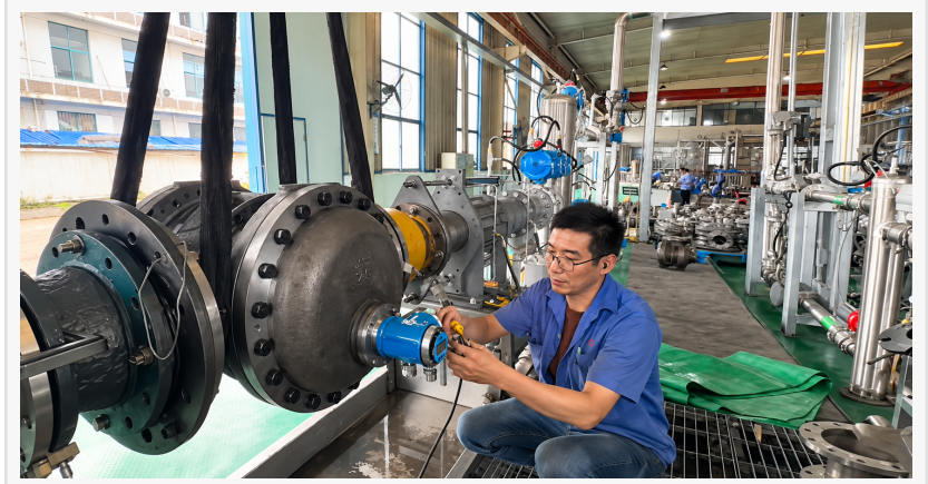
Technician is configuring a large oval gear flow meter in the workshop
