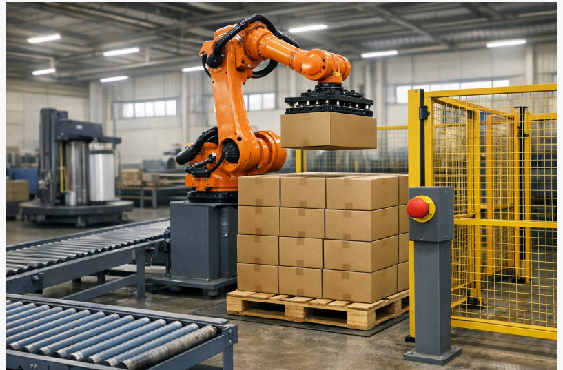
A retrofitted robotic palletising cell at the end of an existing roller conveyor, with yellow safety guarding and an emergency stop beside the pallet station in a Kempton Park packing hall.
